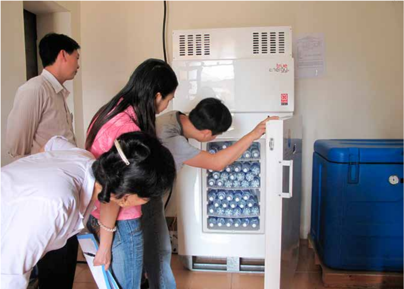
Thanh Ba district , Phu Tho province, Viet Nam: Pilot tests of this solar-powered refrigerator found that the cold chain could be preserved for up to two weeks without electricity. (Photo: Project Optimize/PATH/Hai Le)
