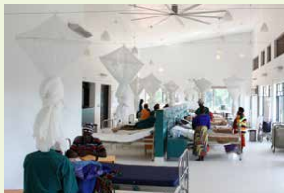
Butaro District Hospital, Rwanda: Patient beds face a window, so healing mothers have a view of nature, while ceiling fans affixed to the high ceilings support cooling and fresh air circulation. (Photos: MASS Design Group)
